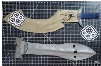
Image 6: Sample weapon controllers with showing detachable fiducials.
